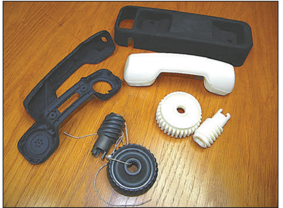
Telephones and gears made in 3D printers compared to the original gears (front). The black phone was done on a high resolution printer, while the white phone was printed on the low resolution printer owned by Seginus.
