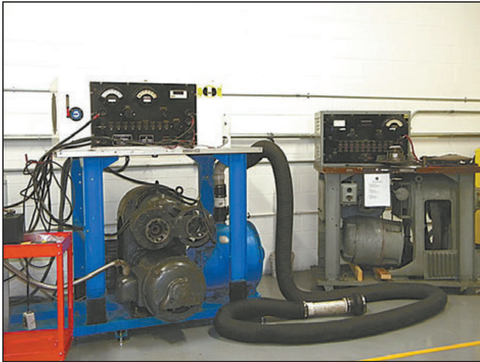
Testing equipment used in the repair process for starter generators.
